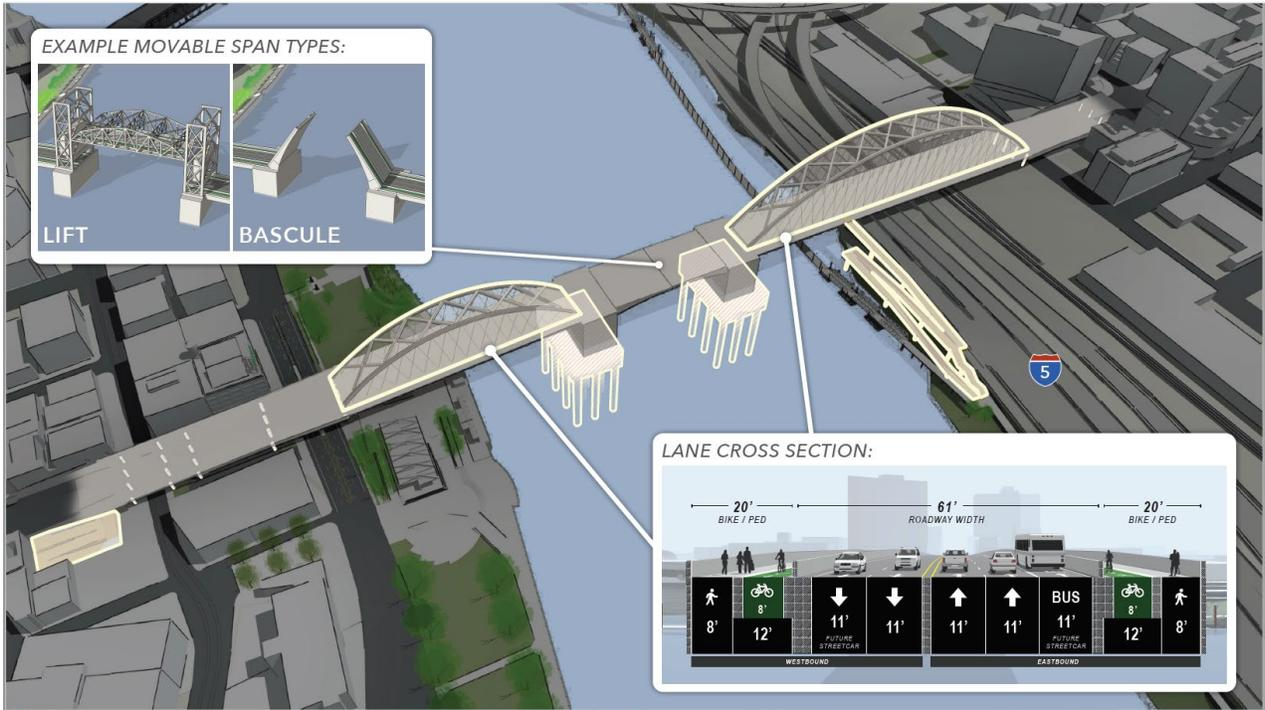
Note: The Draft EIS Long-span Alternative included multiple bridge types for both the east and west approaches. This figure shows only the tied arch option.
