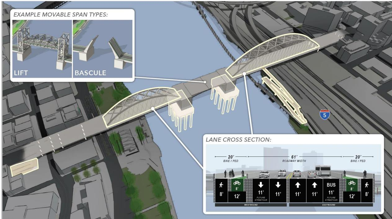
Note: The Draft EIS Long-span Alternative included multiple bridge types for both the east and west approach. This figure shows only the tied arch option.
