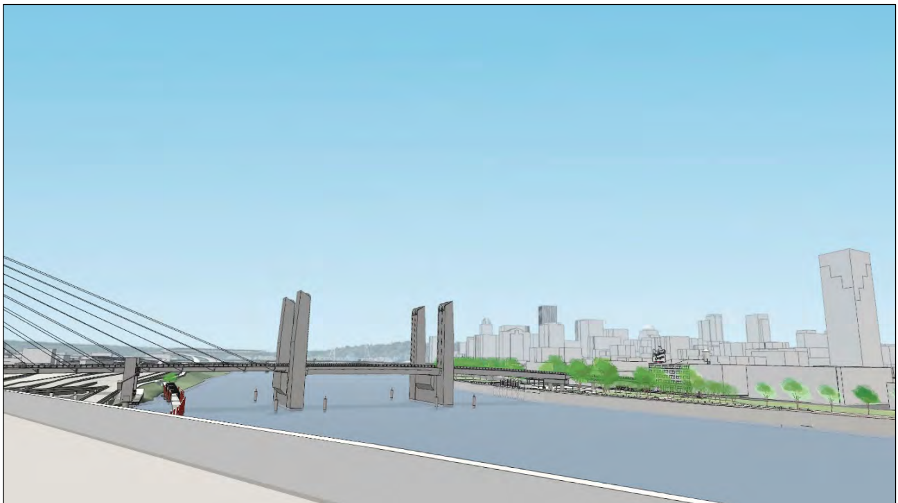
Figure 42: Span Combination 4 (girder west approach, vertical lift central span, cable supported east approach), artist's rendering, view looking southwest (Fat Pencil Studio, 2021).
