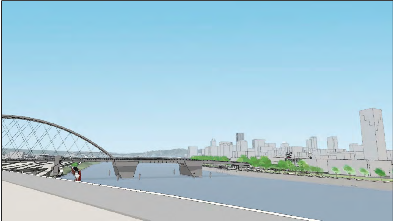
Figure 39: Span Combination 1 (girder west approach, bascule central span, tied arch east approach), artist's rendering, view looking south (Fat Pencil Studio, 2021).
