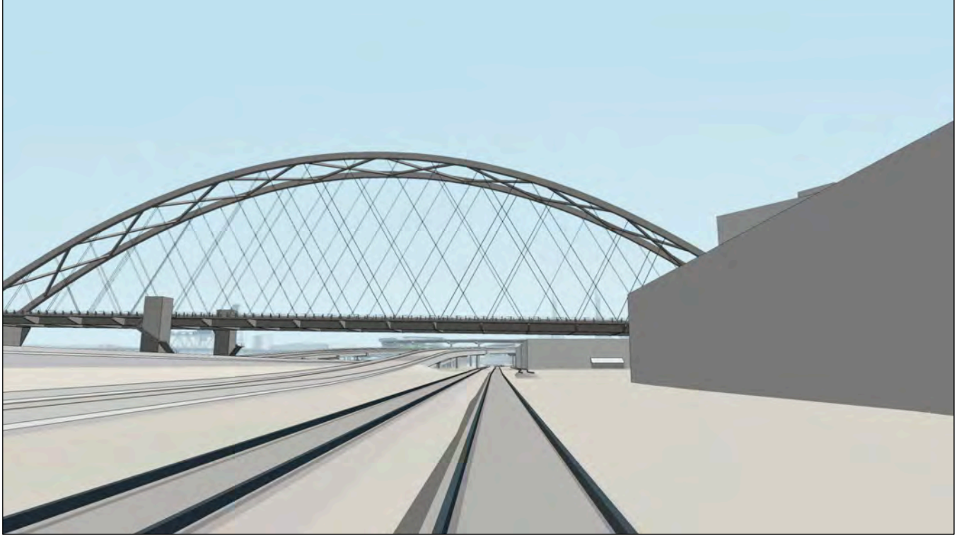
Figure 9. Oregon & California RR (UPRR) alignment looking north toward the Burnside Bridge undercrossing, artist's rendering of proposed new eastern approach with tied-arch structure (Fat Pencil Studio, 2021).
