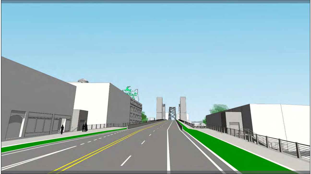
Figure 65: Span Combination 2 (girder west approach, vertical lift central span, tied arch east approach), artist's rendering, view looking east (Fat Pencil Studio, 2021).
