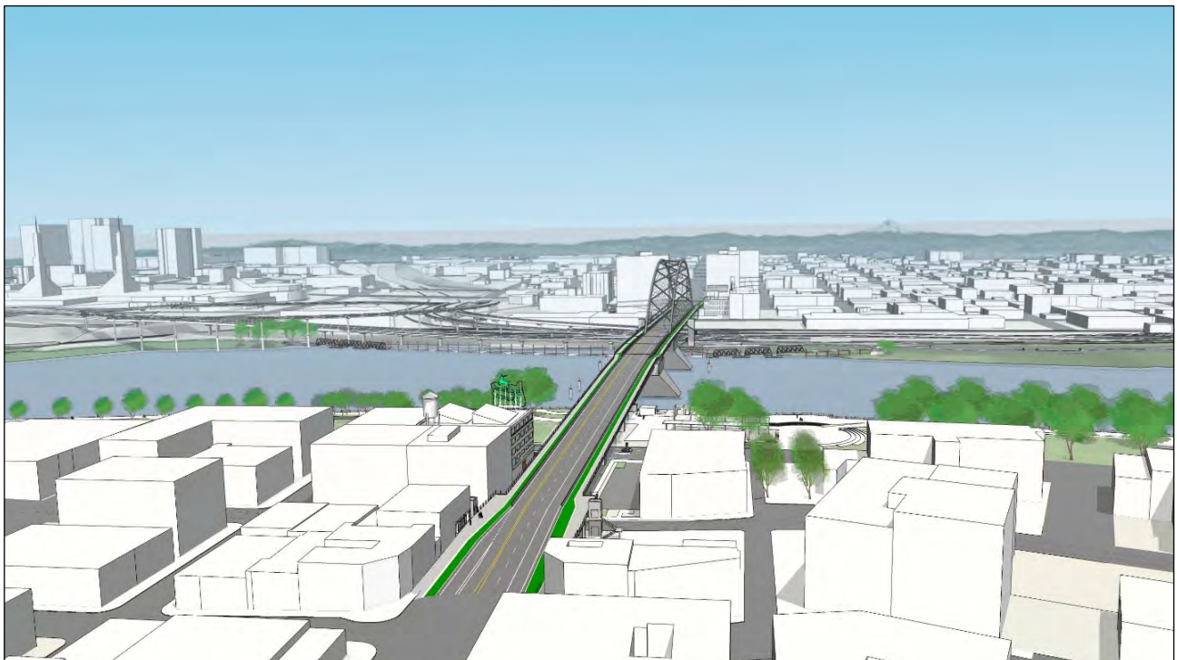
Figure 54: Span Combination 1 (girder west approach, bascule central span, tied arch east approach), artist's rendering, view looking east (Fat Pencil Studio, 2021).
