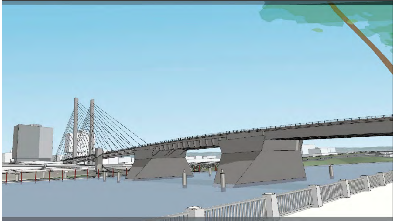
Figure 51: Span Combination 3 (girder west approach, bascule central span, cable supported east approach), artist's rendering, view looking southeast (Fat Pencil Studio, 2021).
