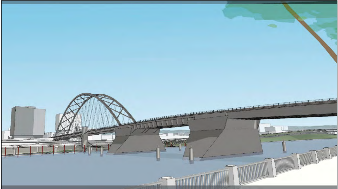
Figure 49: Span Combination 1 (girder west approach, bascule central span, tied arch east approach), artist's rendering, view looking southeast (Fat Pencil Studio, 2021).
